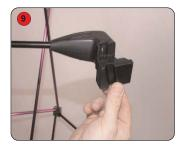
Slide it on with the clip hanging off the back of the light.
