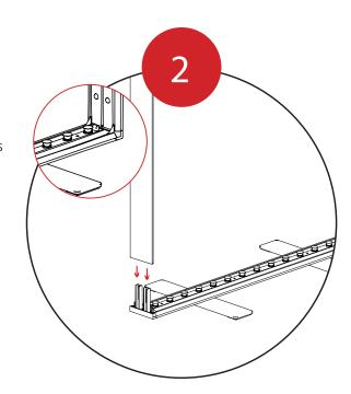
Fit the Side Extrusion Tops ▲ onto the Side Extrusion Bottom ● connectors.
