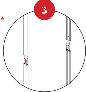
Fit the Top Extrusions together.
