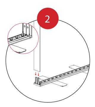
Fit the Side Extrusion Tops
