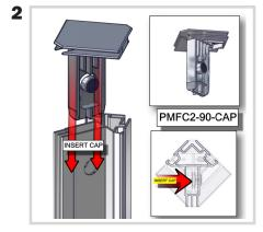
Push down on the snap button on your cap and push it into the top and bottom of the vertical posts until it snaps in place.
