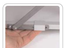
Slide locking tab over pivot arm at base of unit. Repeat for second locking arm.
