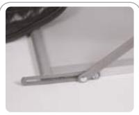
While raising the unit note position of pivot arms. Both pivot arms must rotate through 180 degrees.
