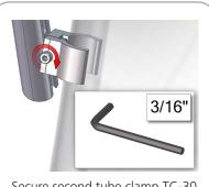
Secure second tube clamp TC-30 around backwall and tighten with 3/16" hex key tool.
