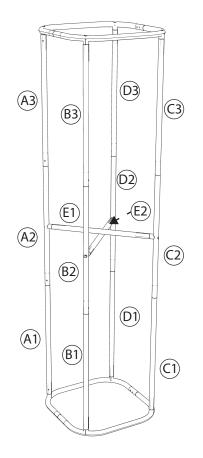
Press button & insert swaged end into receiving end of tubing
