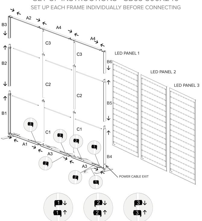
AC POWER CABLE: NO:1 EXTENSION CABLE: NO:2 EXTENSION CABLE: NO:3
