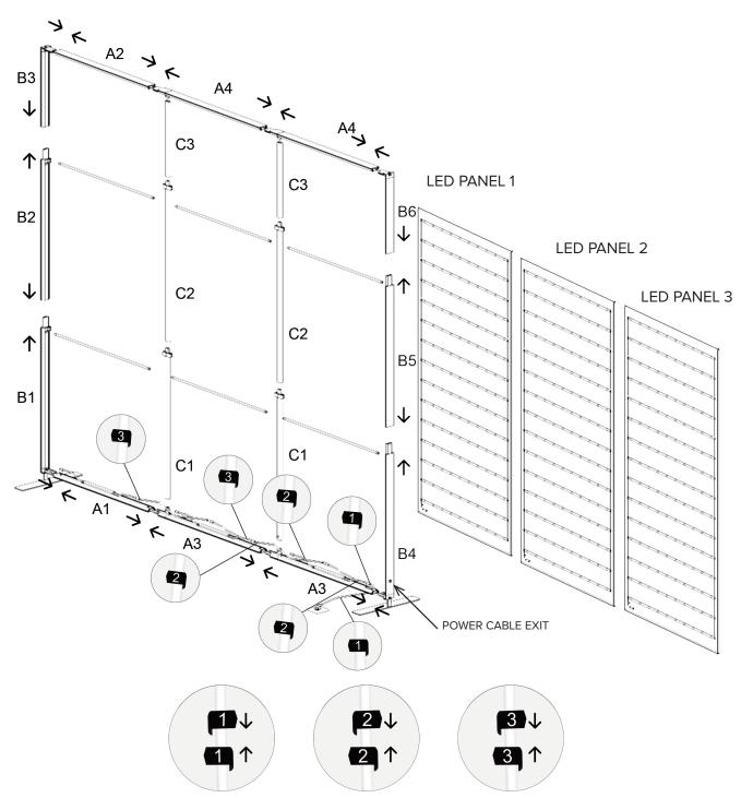
AC POWER CABLE: NO:1 EXTENSION CABLE: NO:2 EXTENSION CABLE: NO:3
