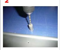
drill the hole through the pole bucket
