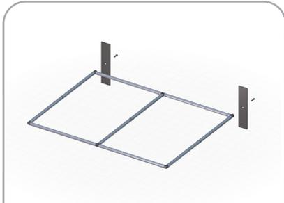
Once frame is connected attach feet. It is best to assemble with frame still laying flat.
