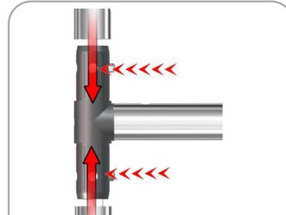
Using TC-30-T to connect frame in the middle at top and bottom.
