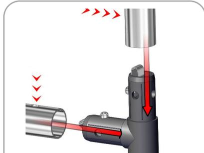
Use TC-30-90B for bottom corners. Connect sides of frame to elbow joint by pressing snap buttons.
