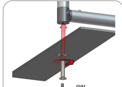
Using provided allen key, secure feet to bottom of frame by screwing bolt.
