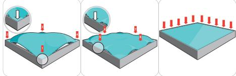
First, insert the silicone edge frame corners into the frame graphic channel (points 1 through 4). Second, insert the silicone edge frame sides into the frame graphic channel (points 5 through 8). Third, push the remaining silicone edge fabric into the frame graphic channel.
