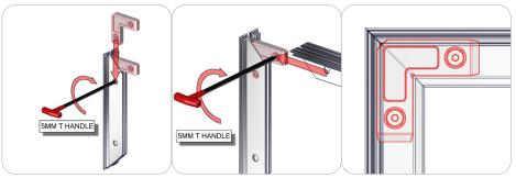
First, insert the corner connector into the extrusion while holding in the lock button. Then, slide the next extrusion onto the same corner connector again holding in the lock button. Finally, use the provided allen key to lock the corner connector in place. Use the allen key tool to press the lock buttons, make quarter turns and do not over tighten the lock buttons.
