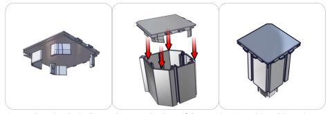
First match up the plastic clips, on the cap to the shape of the extrusion. Second, just slide cap into position.
