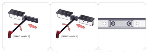
First, insert the in-line connector into the extrusion while holding in the lock button. Then, slide the next extrusion onto the same in-line connector again holding in the lock button. Finally, use the provided allen key to lock the in-line connector in place. Use the allen key tool to turn the lock buttons, make quarter turns and do not over tighten the lock buttons.
