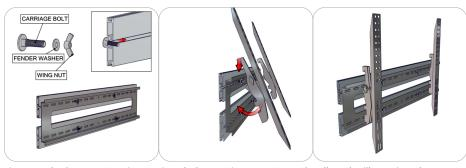
First, attach plate to PS2 using carriage bolts an wing nuts. Second, Follow the illustration above on how to connect TV arms. Last, once arms are attach and fix correctly, then remove them. Its recommend you attach arms to the back of the MONITOR before installing.
