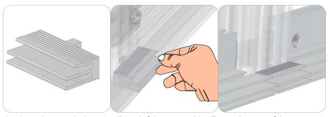
First, insert the spacer in the center channel of the PM2S2. This will cover the space of the voidbetween both PHFC4 extrusions. Second, mover to the desired position needed.
