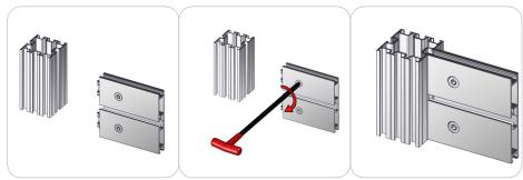
First, insert PS2 camlock into PMS2S side with one channel. a line the parts to your desired locate. Use tool pictured to lock, cam lock in place. Be sure not to over tighten, this could cause damage to parts or extrusions.
