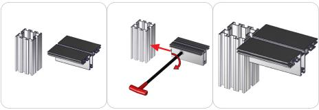
First, insert PHFC4 camlock into PMS2S side with one channel. a line the parts to your desired locate. Use tool pictured to lock ,cam lock in place. Be sure not to over tighten, this could cause damage to parts or extrusions.
