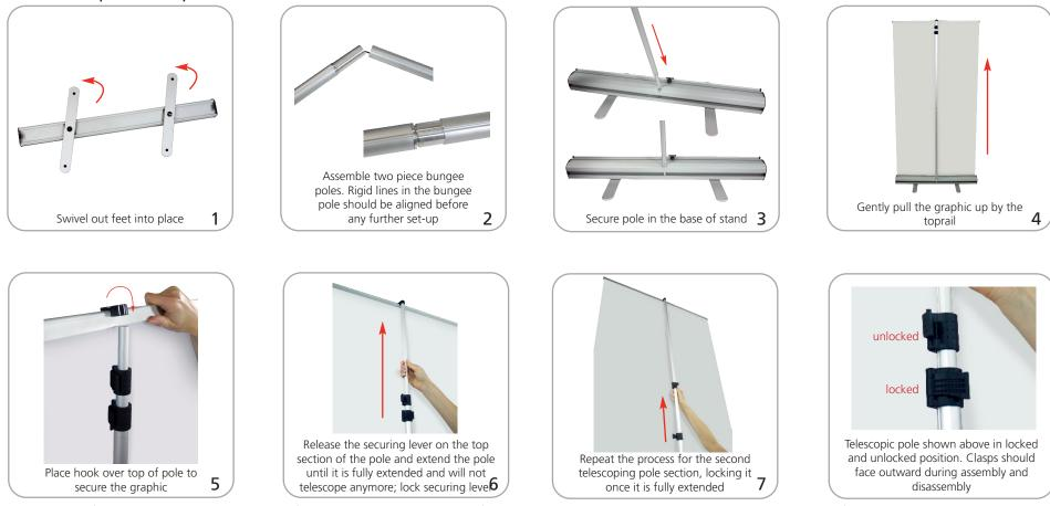
\*To disassemble from maximum height, second section of telescopic pole should be retracted first. Slowly guide the pole down towards the base and repeat with the first pole section.
