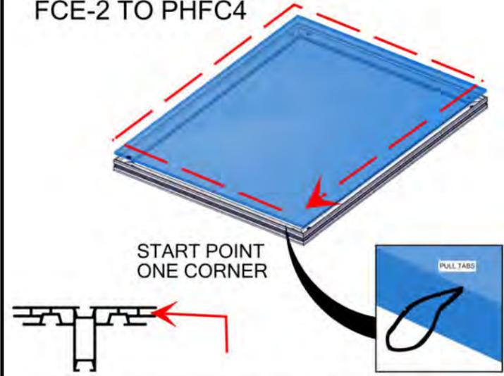
Install graphic by pressing the FCE-2 into the channels of PHFC4 extrusion. To pull graphics out of the channels, use tabs on the front side
