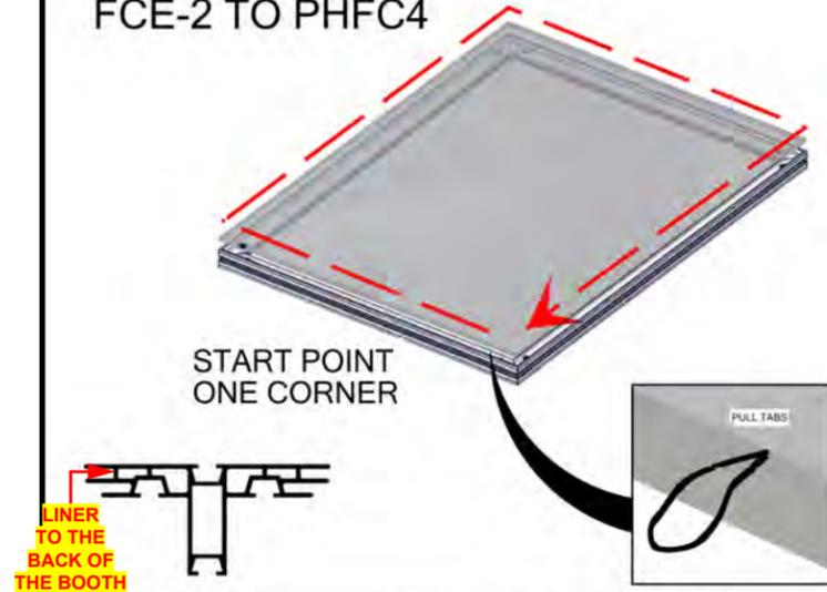
Install liner by pressing the FCE-2 into the channels of PHFC4 extrusion. To pull liner out of the channels, use tabs on the front side
