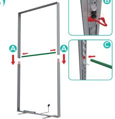
• Place the top half of the extrusion and slide onto the split connector of the bottom half extrusion. Connect LED Wire Connector to LED strips. Install Support Pole on each side of the inner frame.
