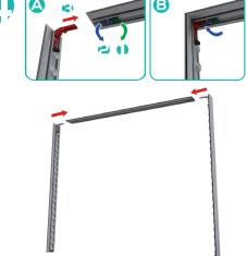
• Slide side extrusions into top extrusion channel. Use latch to press down on the L connector. Then press down the second latch to secure.
