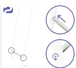
Align the Bottom Support Tube screw holes with holes of the lower leg tubes on each side. Insert the large screws and tighten to secure with allen key.
