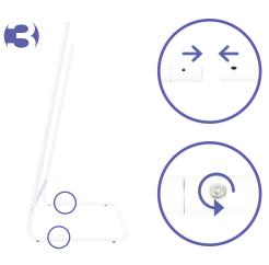
• Connect the Bottom Tube and the bottom Leg Tubes to align holes together. Insert the screws and tighten to secure with allen key.
