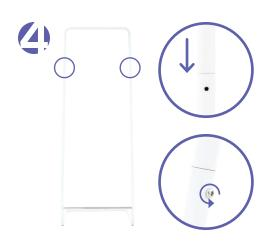
• Insert the Top Tube on top of the Leg Tubes to align holes. Insert the screws and tighten to secure with allen key.
