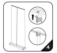
Attach support pole to rear slot of the clamp bar.
