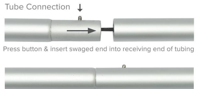
Press button & insert swaged end into receiving end of tubing
