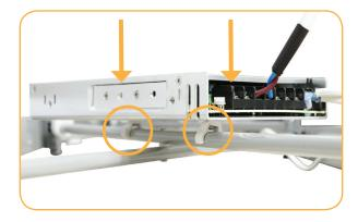
**c.** Place transformers on the bottom of the frame by snapping onto the cross sections.
